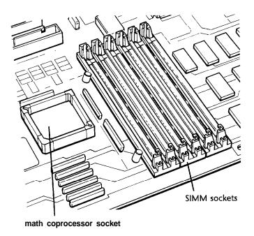
5. The math coprocessor socket is hollow and square, and has a notch in the lower left corner, as shown below.
